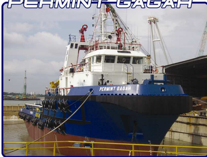
ANCHOR HANDLING TUG SUPPLY VESSEL FIFI 1 BHP 5500 BOLLARD PULL 77 TONNE
